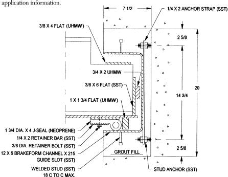
Fabricated stainless steel bulk head, embedded slot
